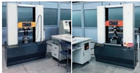
Static stiffness test for ball screw and linear guide
