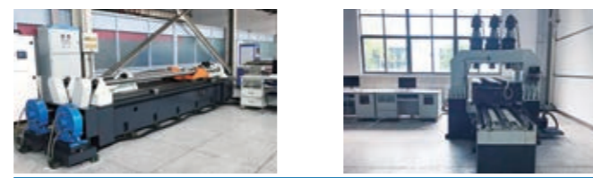
Fatigue life test for ball screw and linear guide
