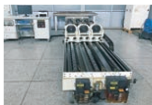
Static stiffness test for ball screw and linear guide
